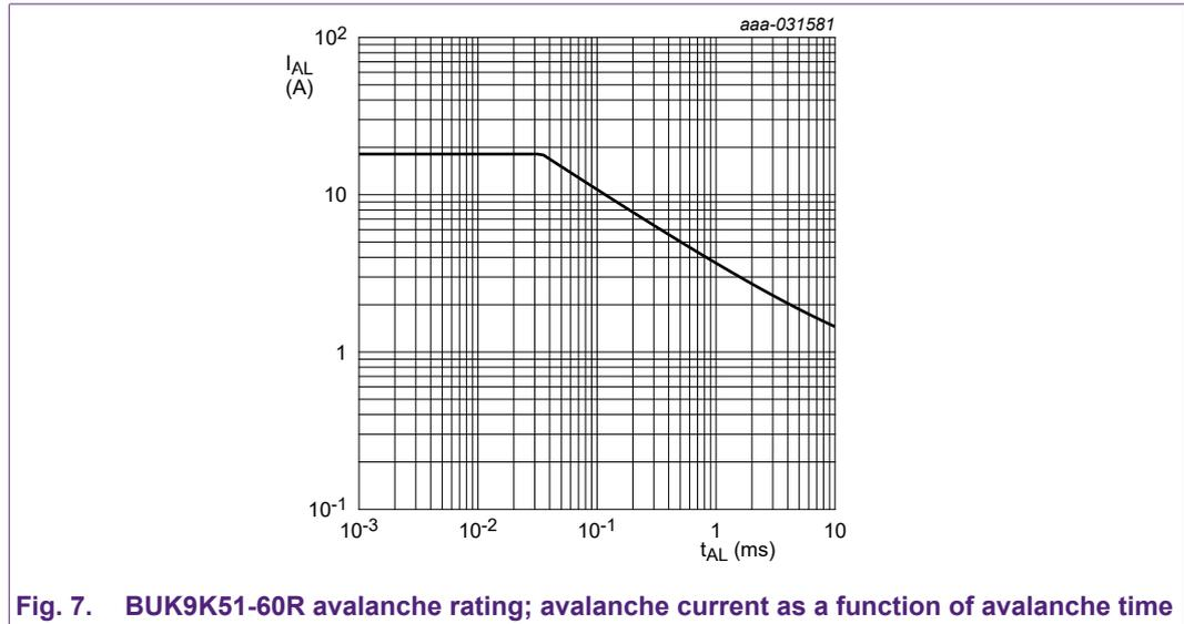
**Fig. 7. BUK9K51-60R avalanche rating; avalanche current as a function of avalanche time**
