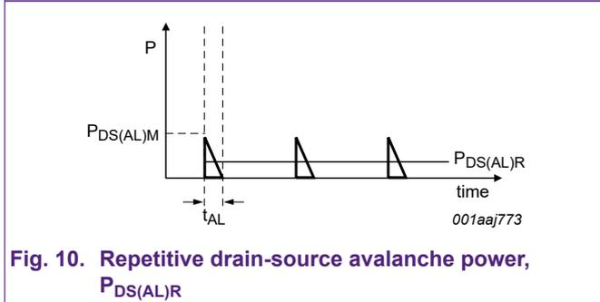
Fig. 10. Repetitive drain-source avalanche power,  $P_{DS(AL)R}$
