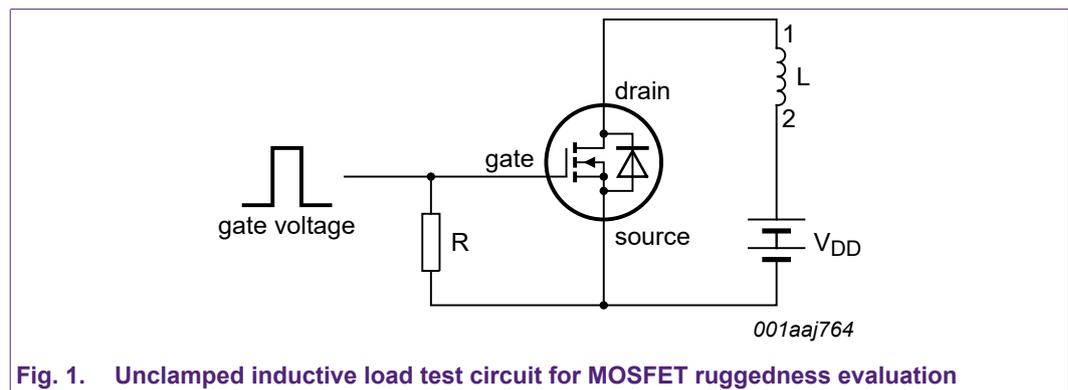
**Fig. 1. Unclamped inductive load test circuit for MOSFET ruggedness evaluation**
