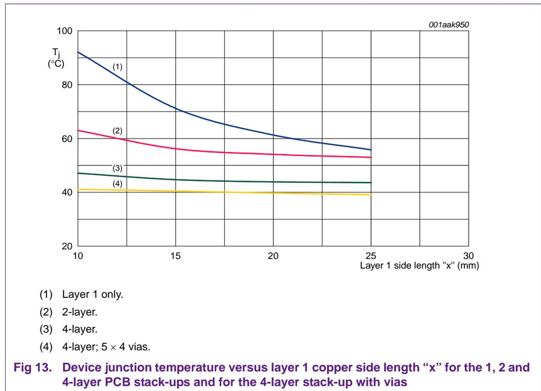
It can be seen that, once vias are added under the device,  $T_j$  becomes almost independent of top copper area, and is approximately 5 °C lower than for the 4-layer stack-up without vias.
