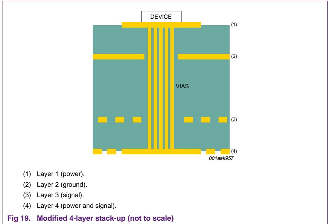
The stack-up of [Figure 19](#) shows the ground plane on layer 2 with the device drain connected to areas on both layer 1 and layer 4, and with the layer 4 copper now also a square of dimensions 15 mm × 15 mm. Layer 3 remains a signal layer. Both MOSFETs are configured in this way, and once again we investigate the influence of separation distance “d” on device  $T_j$ . The results are shown in [Figure 20](#), together with those for the previous analyses.
