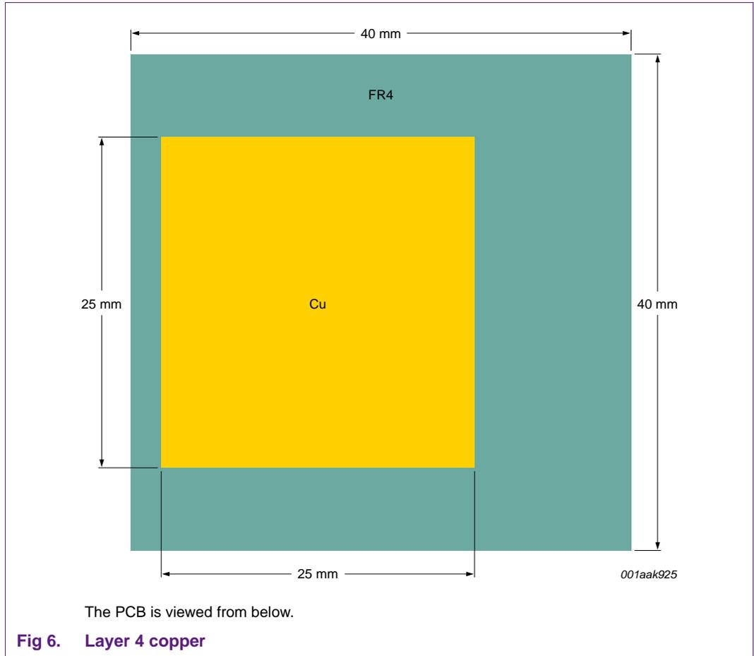
In practical terms this layer might be a ground or power plane, although the device is not electrically connected to this layer.
