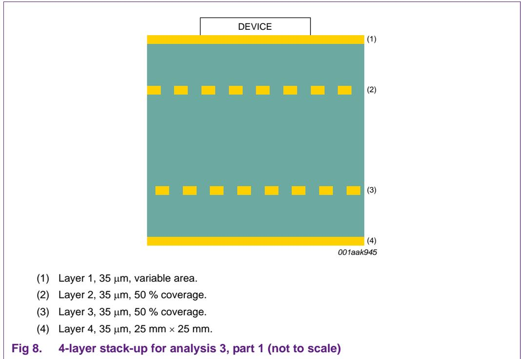
As before, we will carry out simulations for various sizes of layer 1 copper, keeping the other layers constant. The results are shown in [Figure 9](#) together with those from the previous two analyses. Note that there is again no direct connection between the MOSFET and layer 4 plane, and the corresponding circuit topologies would be those shown in [Figure 2 on page 8](#)
