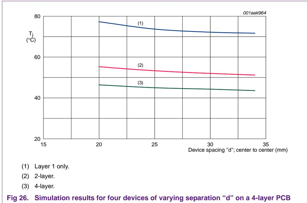
Adding the internal signal layers has resulted in an overall reduction in T<sub>j</sub> of approximately 8 °C.
