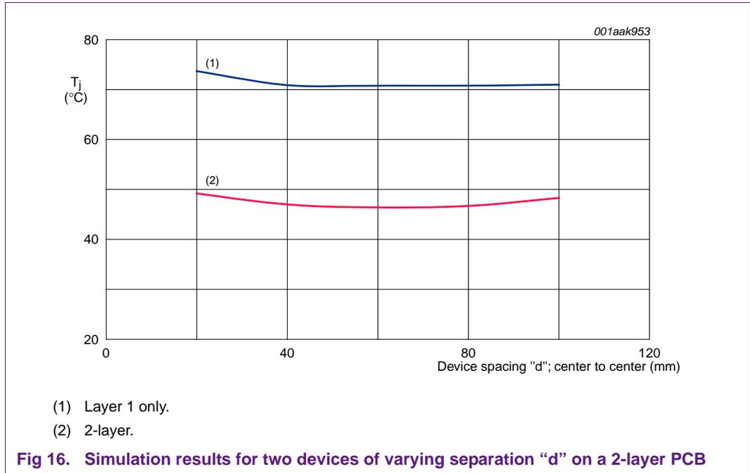
Adding the second copper layer has considerably reduced the junction temperatures of both devices, as one might expect, and temperature still remains largely independent of device separation.
