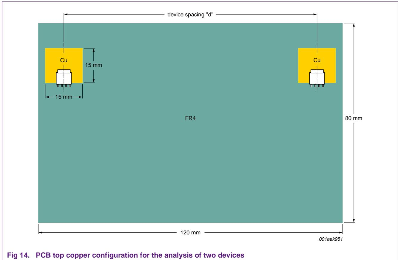
Fig 14. PCB top copper configuration for the analysis of two devices
