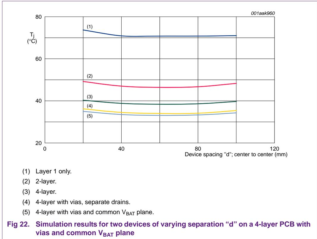
The improvement in thermal performance is practically negligible compared to the previous example (Section 4.4) with independent drain copper areas.
