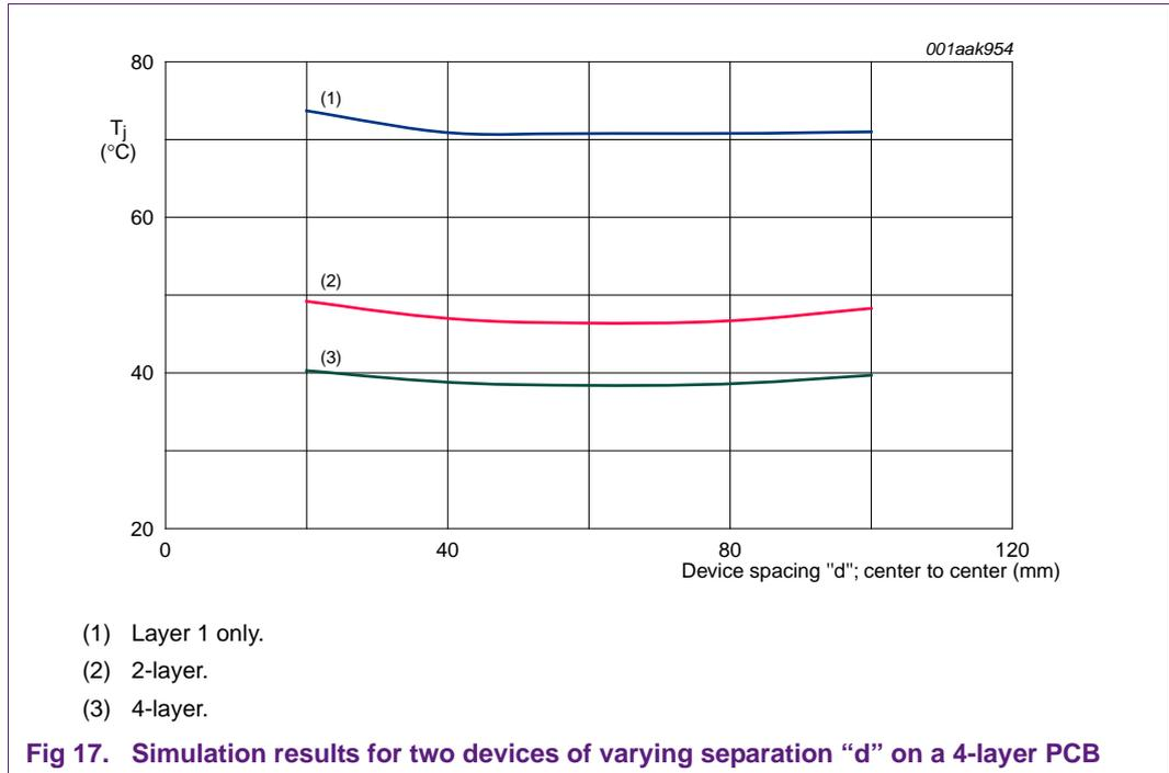
The addition of the two internal layers results in curve of similar shape to the 2-layer stack-up but with an overall reduction in T<sub>j</sub> of approximately 10 °C.
