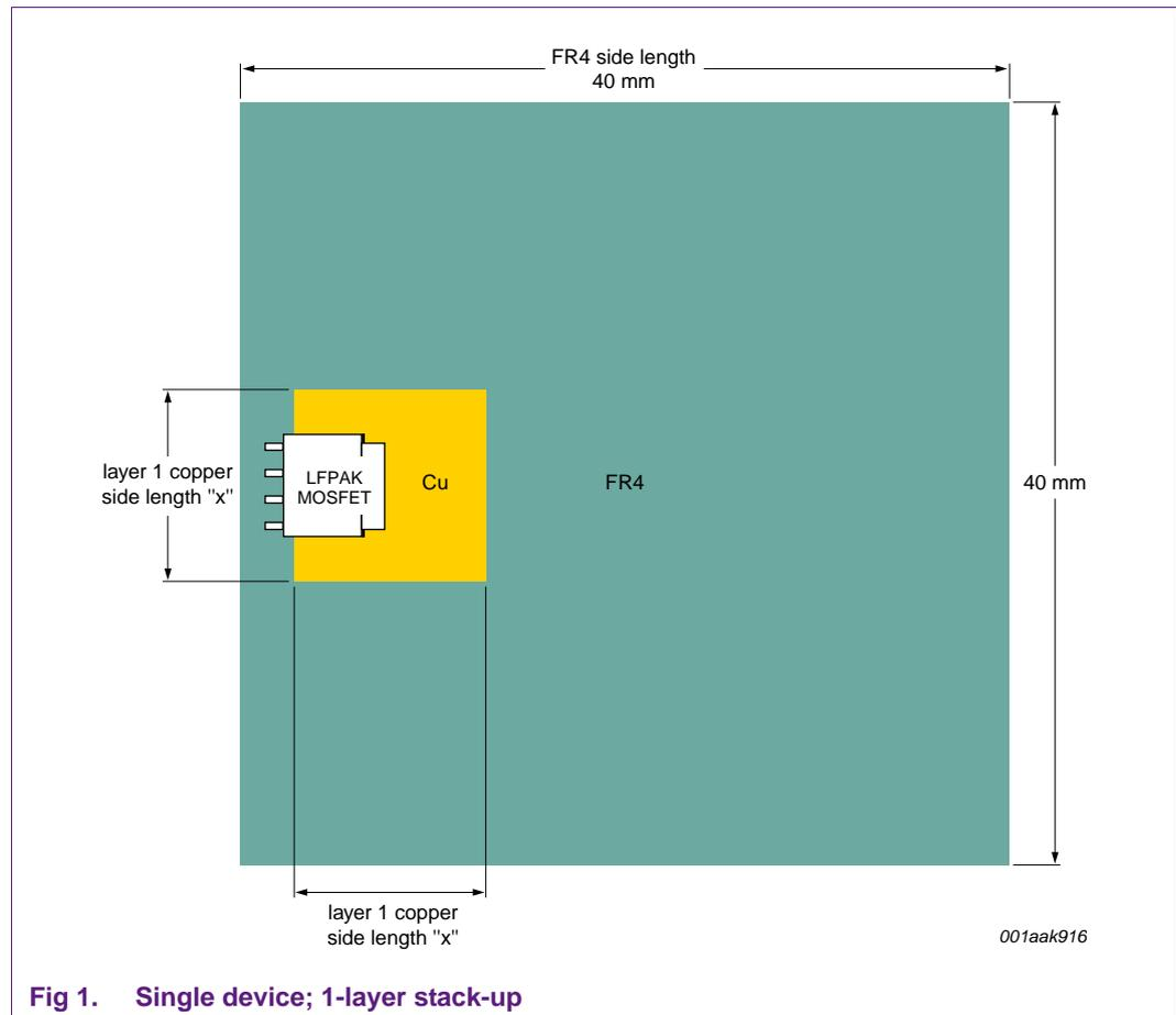
Fig 1. Single device; 1-layer stack-up
