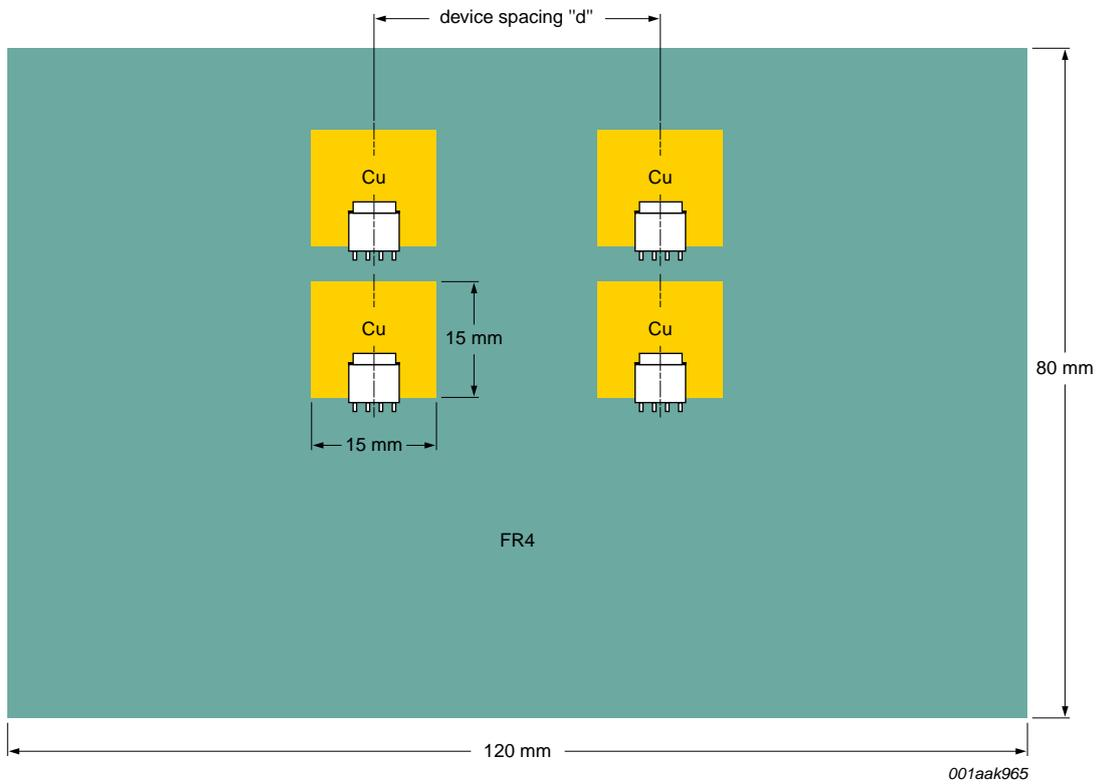
Fig 27. Four devices positioned as two half-bridges configurations
