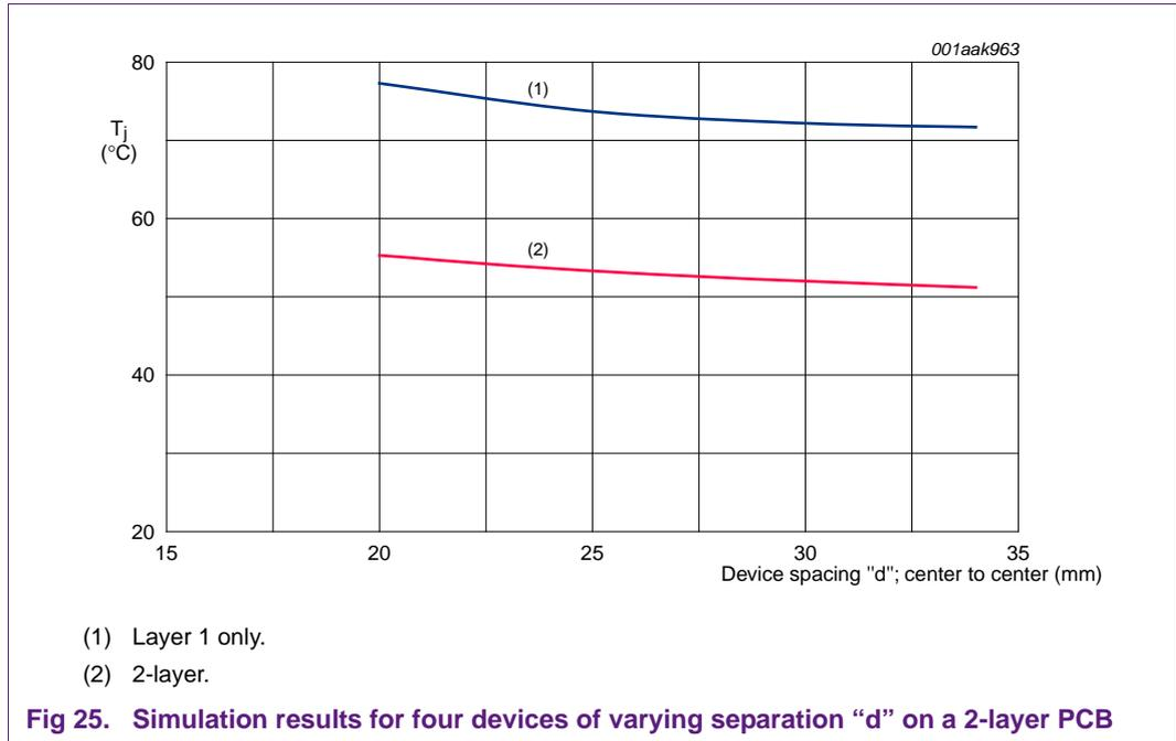
Adding the second copper layer increases the thermal conductivity of the PCB and reduces device temperatures by approximately 20 °C. This is exactly the result we would expect and is in keeping with the results for the one and two-device configurations.
