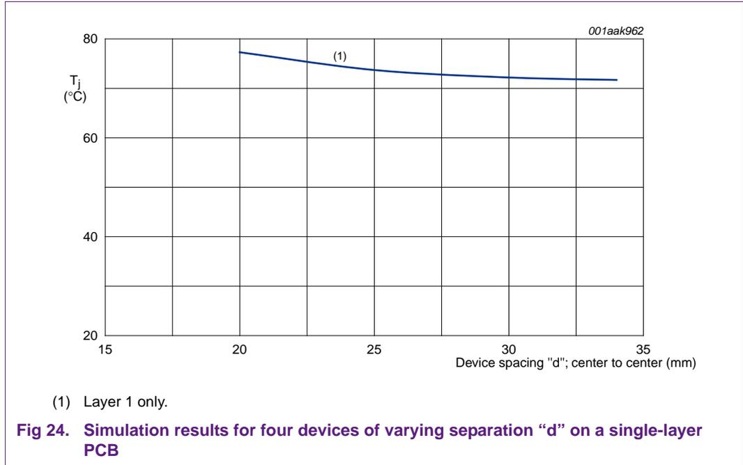
Again, we see the law of diminishing returns exhibited in these results: as the spacing between devices increases, so the curves flattens out. Therefore, increasing the centre – center spacing beyond approximately 30 mm would have little influence on device temperatures.
