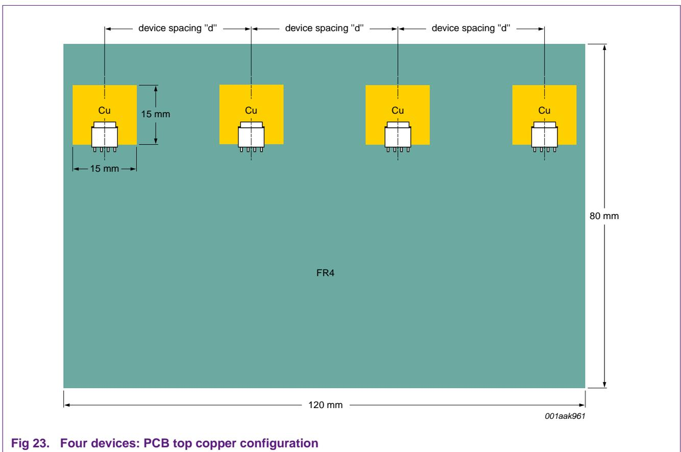
Fig 23. Four devices: PCB top copper configuration
