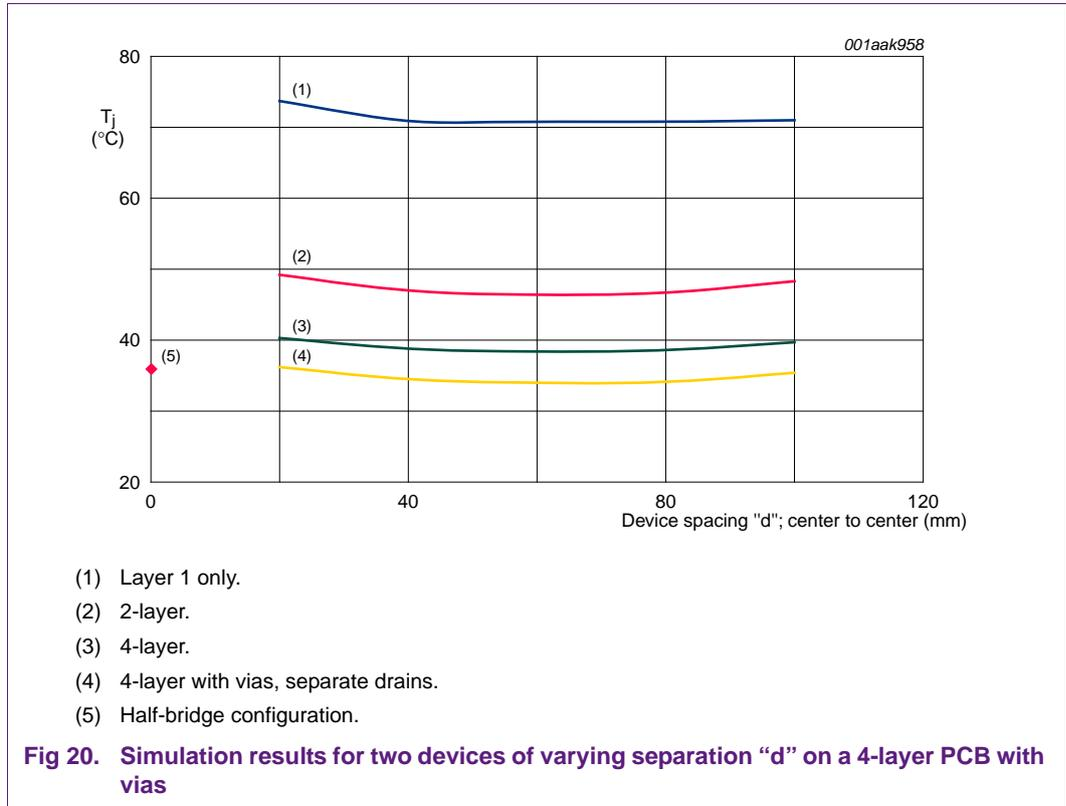
Clearly the addition of vias under the devices results in a further decrease in  $T_j$  even though the layer 4 copper area is reduced. Once again we see that  $T_j$  has little dependence on device spacing.
