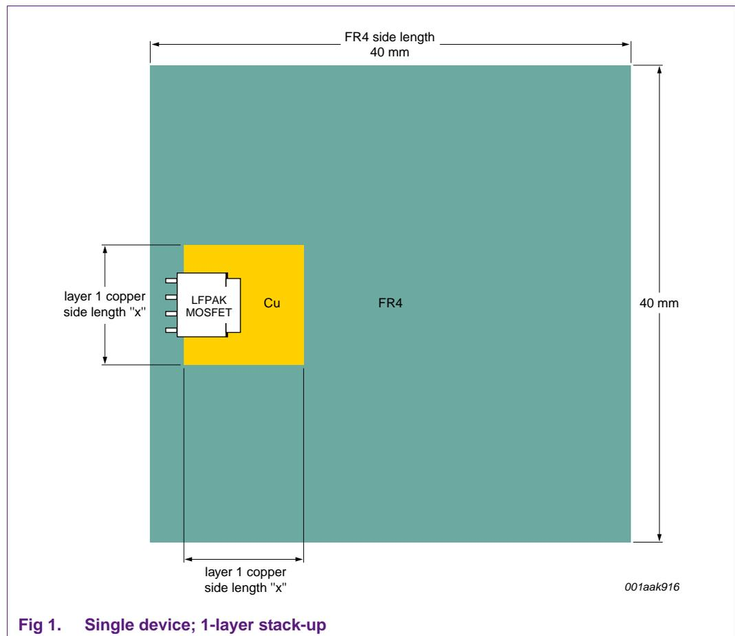
Fig 1. Single device; 1-layer stack-up
