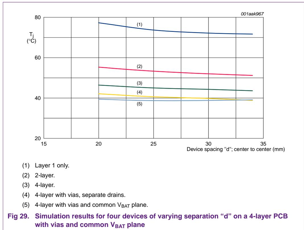
Connecting the four devices does make a small difference to  $T_j$  when the devices are close together, however as “d” increases the effect tends to diminish.
