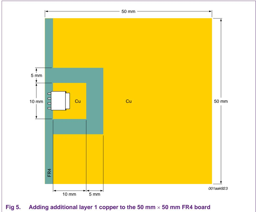
**Fig 5. Adding additional layer 1 copper to the 50 mm × 50 mm FR4 board**
