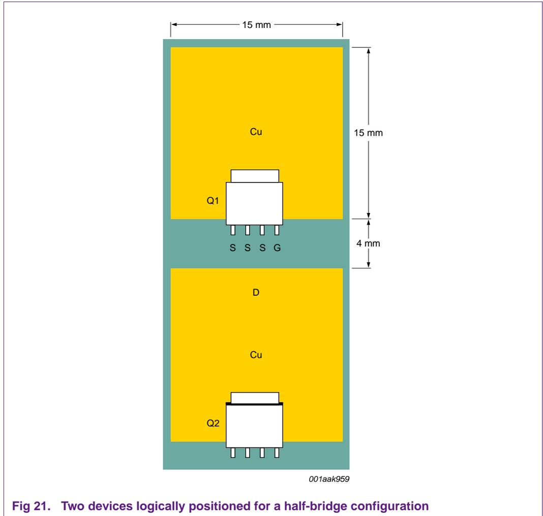
Fig 21. Two devices logically positioned for a half-bridge configuration
