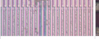
Figure 18. Device 5 after TEOS removal
