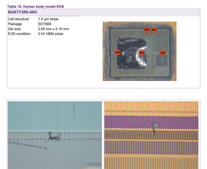
Figure 20. Device 2 after AI, barrier and TEOS etch
