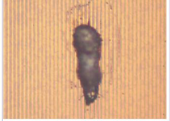
Figure 35. Device 1 upper (orange) hotspot
