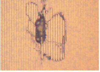
Figure 36. Device 1 lower (orange) hotspot
