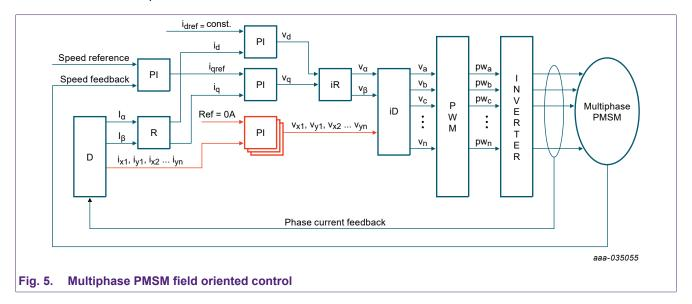
The described so far is identical for three phase and multiphase PMSM's. However, multiphase machines have other currents resulting from the multiphase Decoupling transformations (ix1, iy1, ix2 ... iyn). These are regulated to zero and thus the voltages (vx1, vy1, vx2 ... vyn) are obtained via corresponding PI regulators. These are again subject to inverse Decoupling transformations to contribute to the output voltages. This is illustrated in Fig. 5 with red colour.
