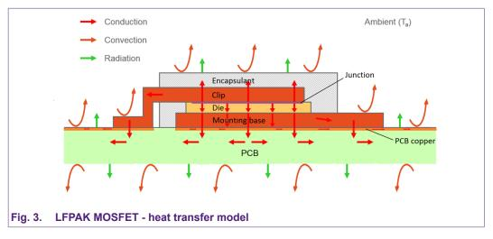
The measured thermal resistance of a MOSFET,  $R_{th(j-a)}$ , depends upon the package size, the material properties and the internal structure of the device. It also depends on the PCB that is used in the test fixture. Modern surface-mount MOSFETs are designed to use the PCB as a heat sink and rely on the copper traces to spread the heat over a large area to assist with cooling.
