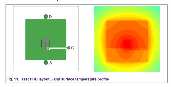
The simulation result gives:  $R_{th(j-a)} = 37.1 \text{ K/W}.$
