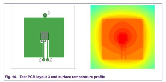
However in a practical working circuit when low R<sub>DSon</sub> MOSFETs are fitted, the drain-source current can reach tens or even hundreds of amperes, and the heat generated in the PCB traces cannot be neglected.
