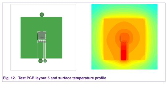
We can deduce from test layouts 4 and 5 that in a practical application involving an LFPAK MOSFET careful consideration must be given to trace thickness and width so that the Joule heating of the current path does not contribute to the heating of the MOSFET.
