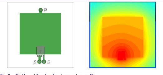
Fig. 8. Test layout 1 and surface temperature profile
