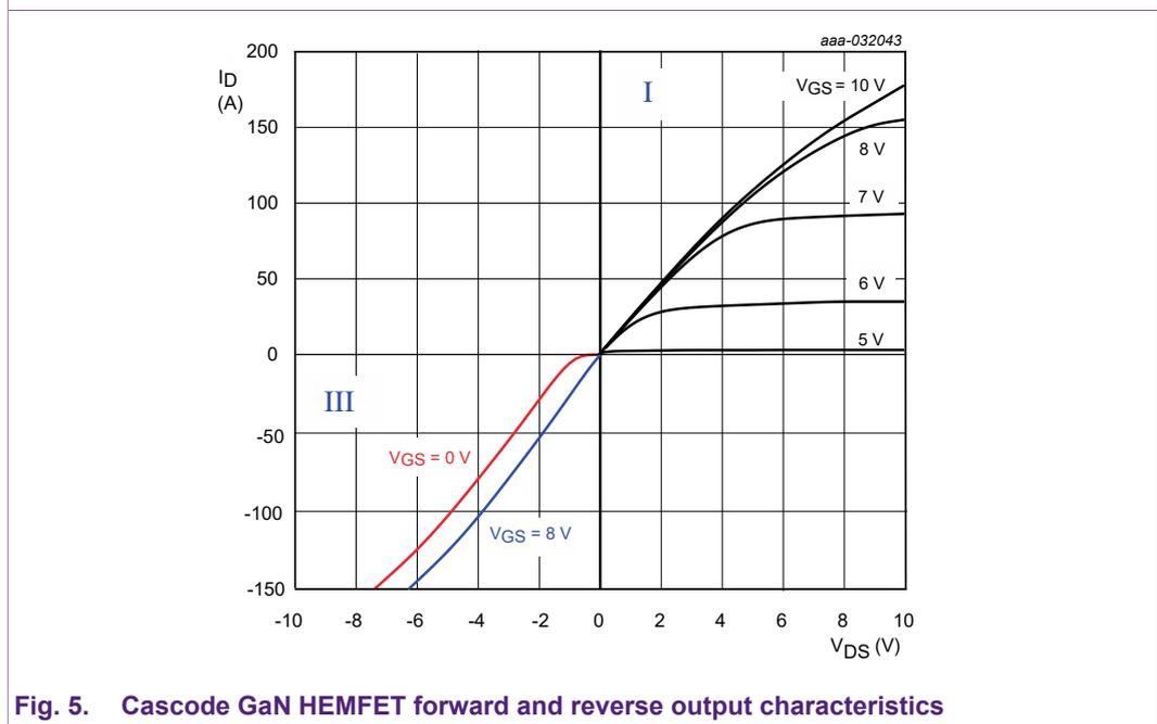
Fig. 5. Cascode GaN HEMFET forward and reverse output characteristics
