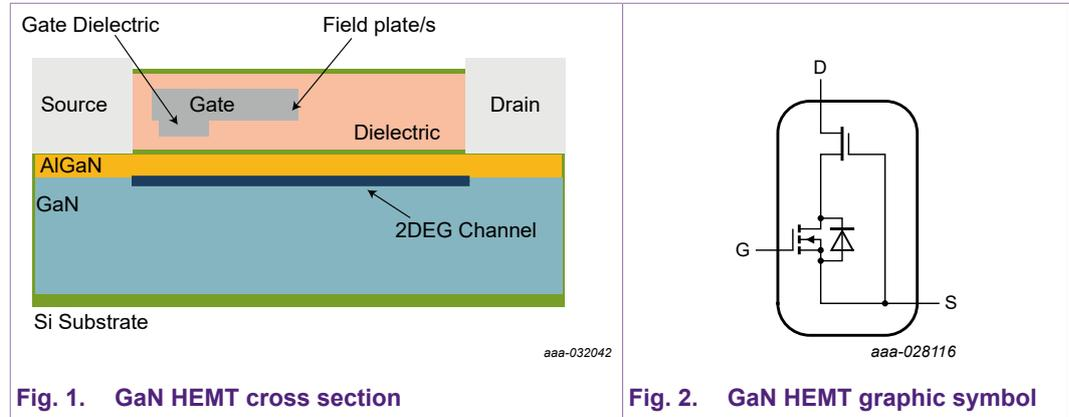
Fig. 1. GaN HEMT cross section
