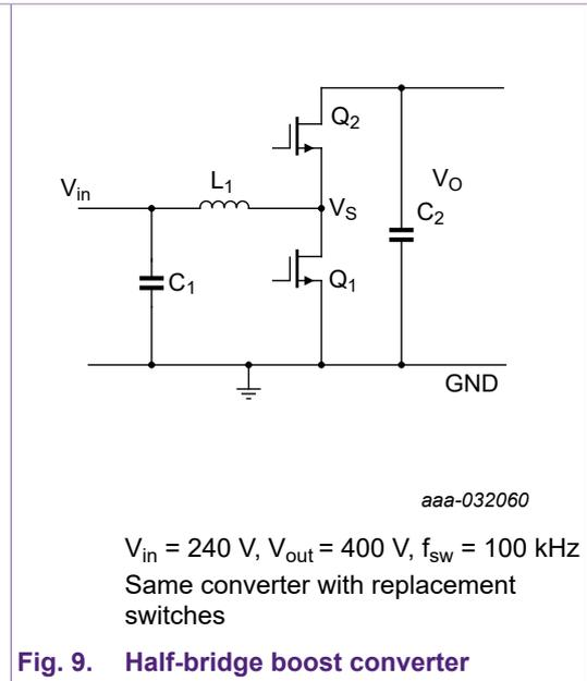
GaN FET losses are significantly lower due to the absence of reverse recovery losses and switching crossover losses. It is possible to achieve near ideal turn on and off losses with  $dV/dt$  of approximately 200 V/ns.
