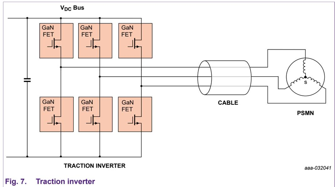
Fig. 7. Traction inverter
