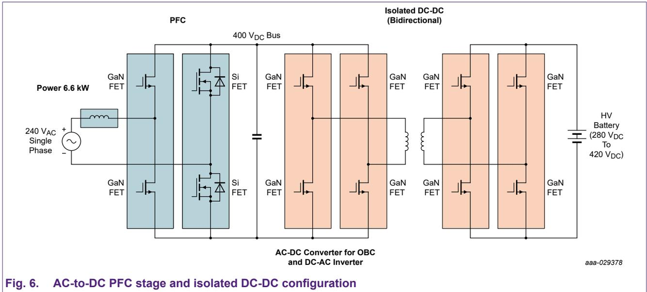
Fig. 6. AC-to-DC PFC stage and isolated DC-DC configuration
