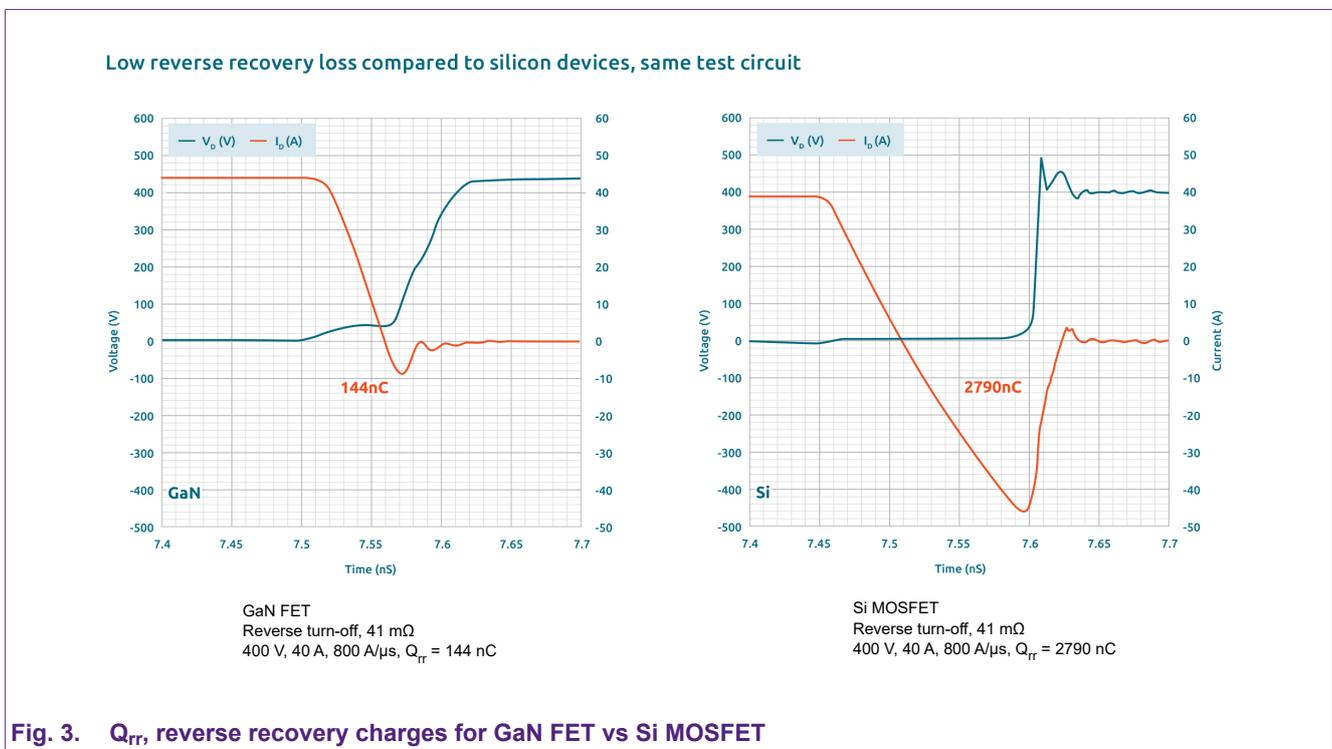
Fig. 3.  $Q_{rr}$ , reverse recovery charges for GaN FET vs Si MOSFET
