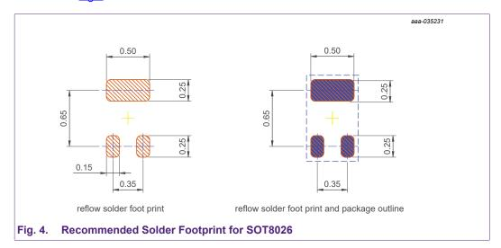
Recommendations for Printed Circuit Board assembly of DSN1006-3 (SOT8026)
