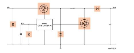
D1 and D2 can be replaced by 2 switch for higher efficiency
