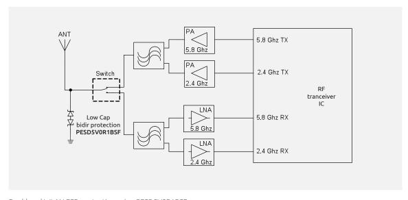
Dual-band WLAN ESD protection using PESD5V0R1BSF
