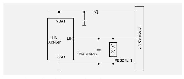
LIN system architecture with a single device to protect the LIN node
