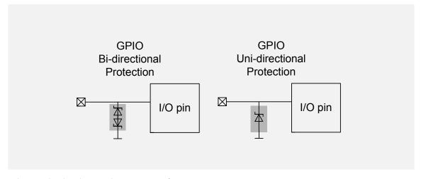
Bidirectional and unidirectional ESD protection for GPIO
