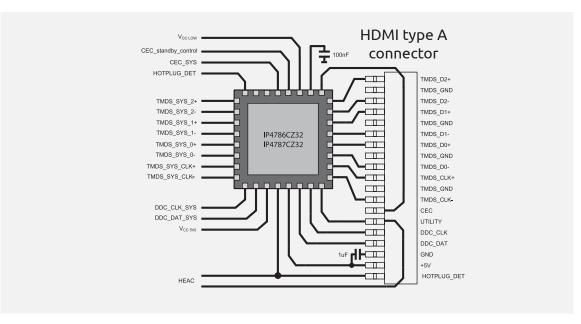
HDMI single-device ESD protection with level shift, showing IP4787CZ32 for receiver and IP4786CZ32 for transmitter applications.
