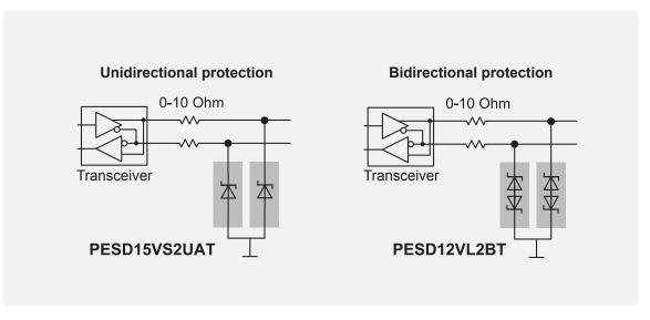
Standard serial port, RS-485, or RS-232 protection can be either unidirectional or bidirectional
