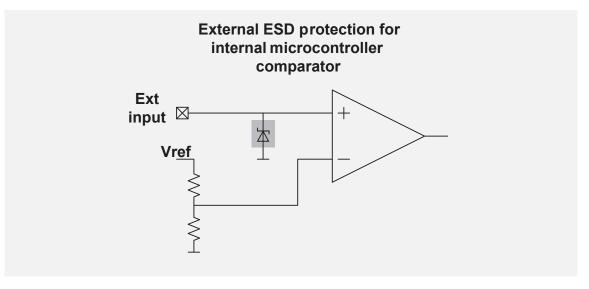
Unidirectional, low-voltage comparator ESD protection
