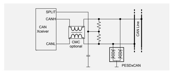
CAN system architecture with a single device to protect the CAN node
