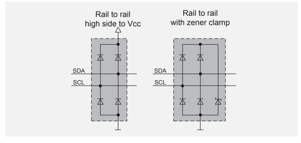
I<sup>2</sup>C protection two rail-to-rail configurations that minimize capacitive line loading
