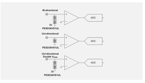
Analog I/O protection using the PESD36VS1UL with single or multiple devices
