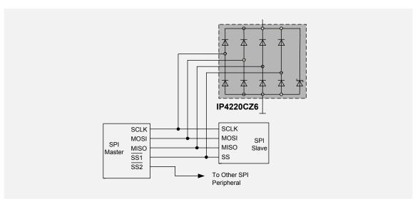
SPI protection showing a single device with a four-line, rail-to-rail diode
