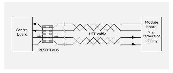
In LVDS systems, the PESD1LVDS provides ultra high-speed ESD protection that is fully AEC-Q101 compliant
