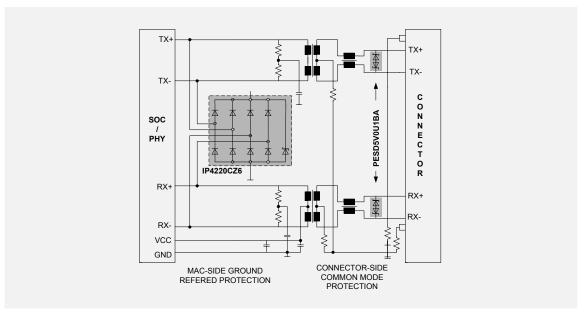
10/100 ESD protection, with ground-referred protection on the MAC side and Common mode protection on the connector side
