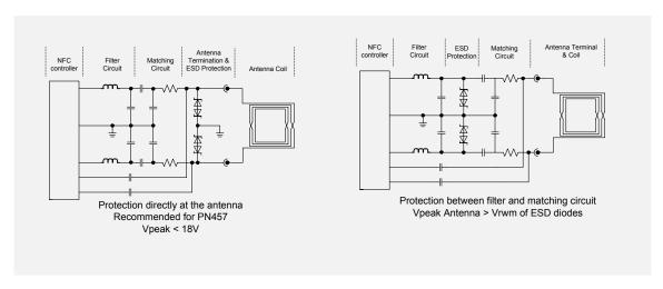
NFC protection can reside at the antenna or between the filter and the matching circuit
