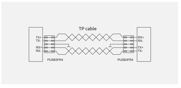
General high-speed differential mode signaling line ESD protection (actual data rate influences device choice)
