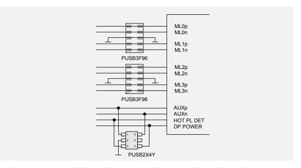
DisplayPort ESD protection with high-speed lines protected with PUSB3F96 and low-speed lines with PUSB2X4Y
