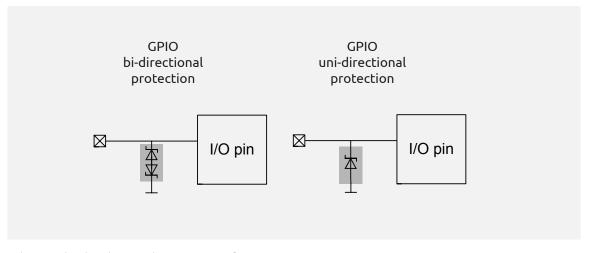
Bidirectional and unidirectional ESD protection for GPIO
