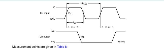
$V_{\text{OL}}$  and  $V_{\text{OH}}$  are typical voltage output levels that occur with the output load.
