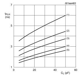
c. LOW to HIGH propagation delay (An to Bn); V<sub>CC(A)</sub> = 2.5 V
