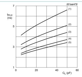
a. LOW to HIGH propagation delay (An to Bn);  $V_{CC(A)}$  = 1.2 V
