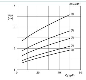
a. LOW to HIGH propagation delay (An to Bn); V<sub>CC(A)</sub> = 1.8 V
