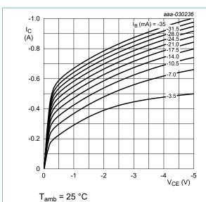
Fig. 24. BC806-25H-Q: Collector current as a function of collector-emitter voltage; typical values
