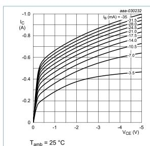
Fig. 12. BC806-16H-Q: Collector current as a function of collector-emitter voltage; typical values
