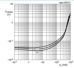
Fig. 20. BC806-25H-Q: Base-emitter saturation voltage
