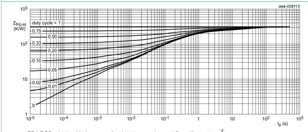
FR4 PCB; single-sided copper; tin-plated; mounting pad for collector 1 cm<sup>2</sup>
