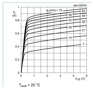
Fig. 12. BC816-16H-Q: Collector current as a function of collector-emitter voltage; typical values
