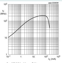
$f = 100 \text{ MHz}; V_{CE} = 5 \text{ V}$  $T_{amb} = 25 \text{ }^{\circ}\text{C}$
