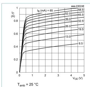
Fig. 24. BC816-25H-Q: Collector current as a function of collector-emitter voltage; typical values
