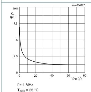
Fig. 14. BC816-16H-Q: Collector capacitance as a function of collector-base voltage; typical values
