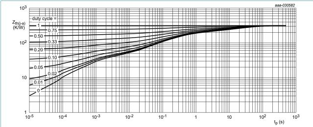
FR4 PCB; single-sided 35 µm copper, standard footprint
