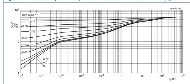
FR4 PCB, 4-layer copper, tin-plated; mounting pad for collector 1 cm<sup>2</sup>
