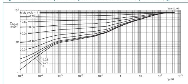
FR4 PCB, single-sided copper, tin-plated; mounting pad for collector 6 cm<sup>2</sup>
