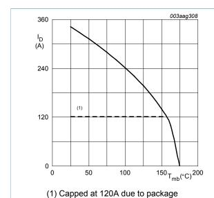
Continuous drain current as a function of Fig. 1. mounting base temperature
