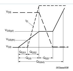
Fig. 13. Gate charge waveform definitions
