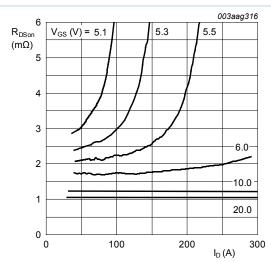
$T_i = 25 \,^{\circ}\text{C}; t_p = 300 \,\mu\text{s}$
