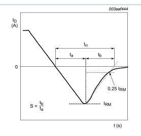
Fig. 17. Reverse recovery timing definition
