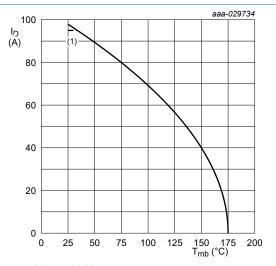
$V_{GS} \ge 10 \text{ V}$  (1) 95A continuous current has been successfully demonstrated during application tests. Practically the current will be limited by PCB, thermal design and operating temperature.
