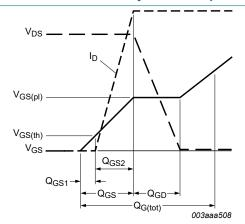
Fig. 14. Gate charge waveform definitions
