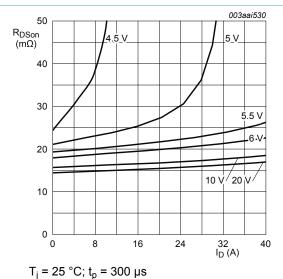
Fig. 11. Drain-source on-state resistance as a function
