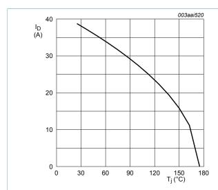
Fig. 1. Continuous drain current as a function of mounting base temperature
