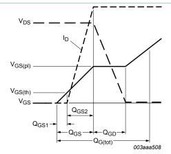
Fig. 14. Gate charge waveform definitions
