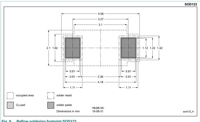
**Reflow soldering footprint SOD123**
