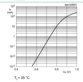
Fig. 3. Forward current as a function of forward voltage; typical values (BZT52-B6V8)
