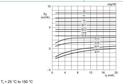
Fig. 7. Temperature coefficient as a function of working current; typical values (BZT52-B4V7 to BZT52-B12)
