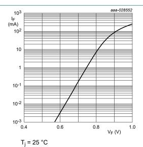
Fig. 4. Forward current as a function of forward voltage; typical values (BZT52-B7V5)
