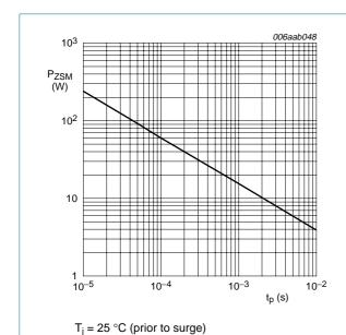
Fig 2. Non-repetitive peak reverse power dissipation as a function of pulse duration; maximum
