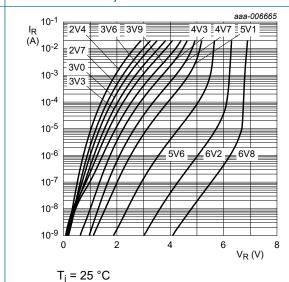
Fig. 8. Reverse current as a function of reverse voltage; typical values (BZX585-B/C2V4 to BZX585-B/C6V8)
