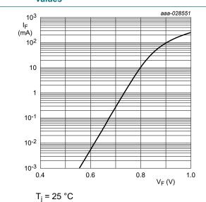
Fig. 3. Forward current as a function of forward voltage; typical values (BZX585-B/C6V8)
