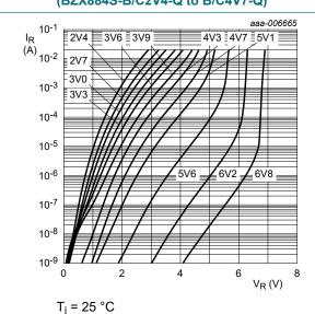
Fig. 7. Reverse current as a function of reverse voltage; typical values (BZX884S-B/C2V4-Q to BZX884S-B/C6V8-Q)
