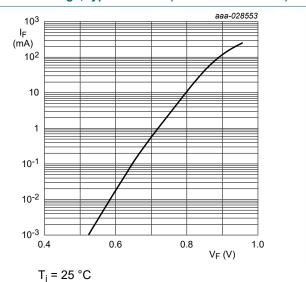
Fig. 4. Forward current as a function of forward voltage; typical values (BZX884S-B/C75-Q)
