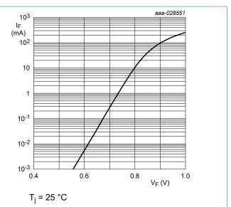
Fig. 2. Forward current as a function of forward voltage; typical values (BZX884S-B/C6V8-Q)
