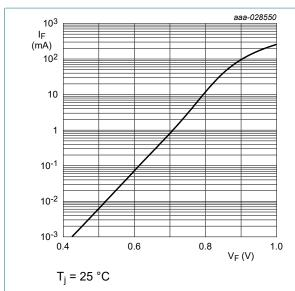
Fig. 1. Forward current as a function of forward voltage; typical values (BZX884S-B/C2V4-Q)
