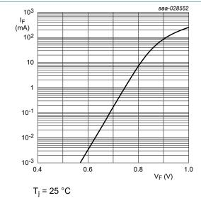
Fig. 3. Forward current as a function of forward voltage; typical values (BZX884S-B/C7V5-Q)
