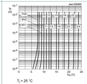
Fig. 8. Reverse current as a function of reverse voltage; typical values (BZX884S-B/C7V5-Q to BZX884S-B/C24-Q)
