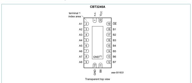
(1) This is not a ground pin. There is no electrical or mechanical requirement to solder the pad. In case soldered, the solder land should remain floating or connected to GND.
