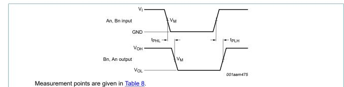
Logic levels:  $V_{OL}$  and  $V_{OH}$  are typical output voltage levels that occur with the output load.
