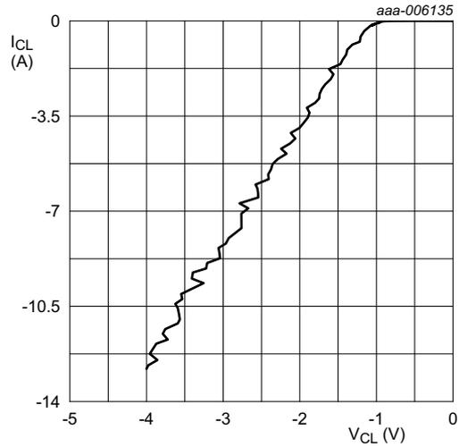
Pin A2;  $t_p = 100$  ns; Transmission Line Pulse (TLP)
