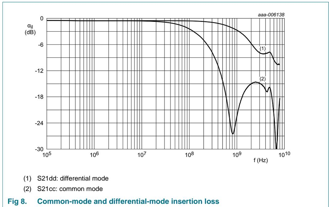
Fig 8. Common-mode and differential-mode insertion loss
