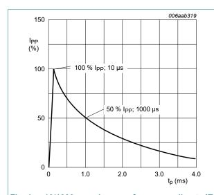
Fig. 1. 10/1000 µs pulse waveform according to IEC 61643-321
