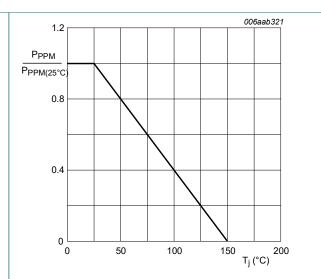
Fig. 4. Relative variation of rated peak pulse power as a function of junction temperature; typical values
