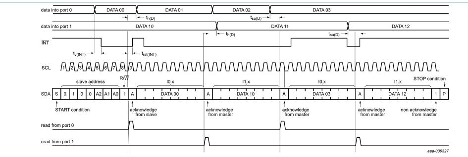
**Remark:** Transfer of data can be stopped at any moment by a STOP condition. When this occurs, data present at the latest acknowledge phase is valid (output mode). It is assumed that the command byte has previously been set to '00h' (read input port register).
