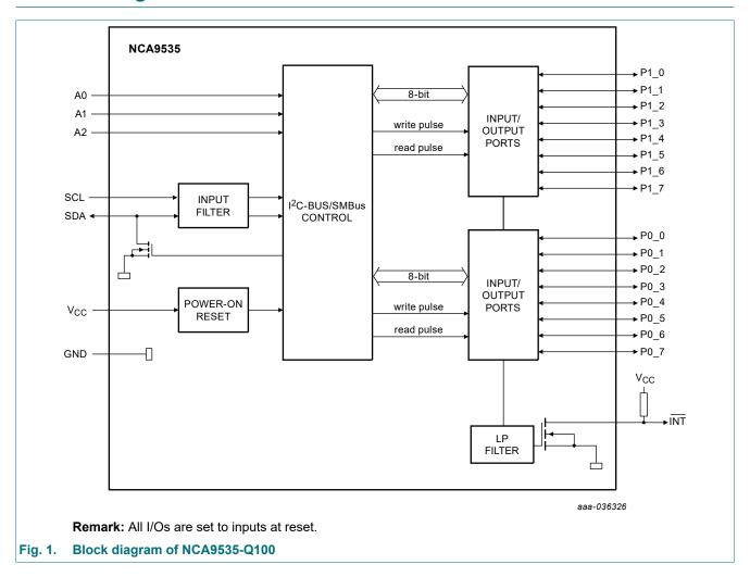
Low-voltage 16-bit I<sup>2</sup>C and SMBus low-power I/O expander with interrupt output and configuration registers
