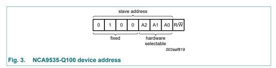
A2, A1 and A0 are the hardware address package pins and are held to either HIGH (logic 1) or LOW (logic 0) to assign one of the eight possible slave addresses. The last bit of the slave address ( $R/\overline{W}$ ) defines the operation (read or write) to be performed. A HIGH (logic 1) selects a read operation, while a LOW (logic 0) selects a write operation.
