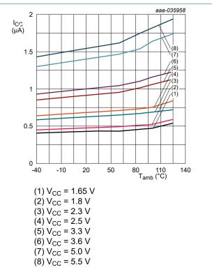
Fig. 18. Supply current versus ambient temperature
