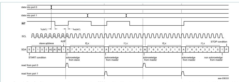
**Remark:** Transfer of data can be stopped at any moment by a STOP condition. When this occurs, data present at the latest acknowledge phase is valid (output mode). It is assumed that the command byte has previously been set to '00h' (read input port register).
