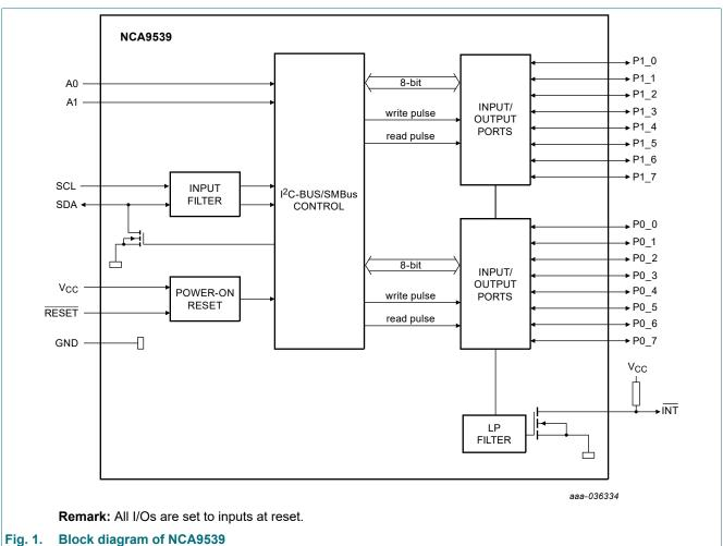
Low-voltage 16-bit I<sup>2</sup>C and SMBus low-power I/O expander with interrupt output, reset pin and configuration registers
