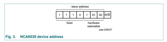
A1 and A0 are the hardware address package pins and are held to either HIGH (logic 1) or LOW (logic 0) to assign one of the four possible slave addresses. The last bit of the slave address ( $R/\overline{W}$ ) defines the operation (read or write) to be performed. A HIGH (logic 1) selects a read operation, while a LOW (logic 0) selects a write operation.
