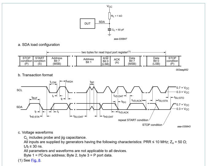
Fig. 25. I<sup>2</sup>C-bus interface load circuit and voltage waveforms
