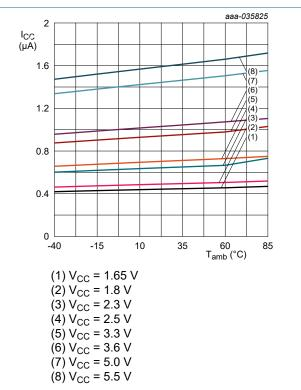
Fig. 18. Supply current versus ambient temperature
