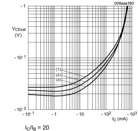
(1) T<sub>amb</sub> = 100 °C (2) T<sub>amb</sub> = 25 °C (3) T<sub>amb</sub> = -55 °C
