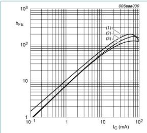
V<sub>CE</sub> = 5 V (1) T<sub>amb</sub> = 150 °C (2) T<sub>amb</sub> = 25 °C (3) T<sub>amb</sub> = -40 °C
