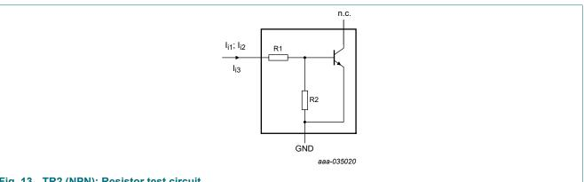
Fig. 13. TR2 (NPN): Resistor test circuit
