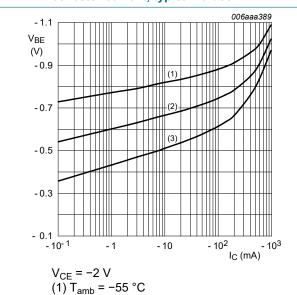
Fig. 3. TR1 (PNP): Base-emitter voltage as a function of collector current; typical values
