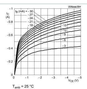
Fig. 2. TR1 (PNP): Collector current as a function of collector-emitter voltage; typical values
