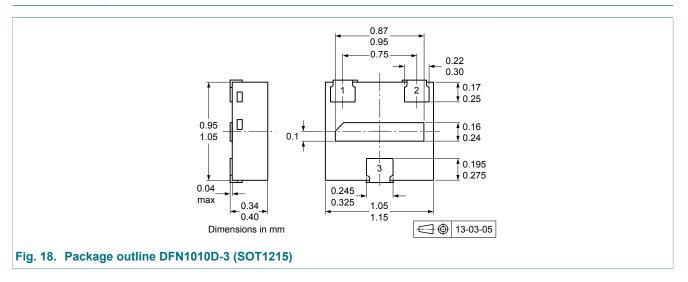
60 V, 1 A PNP low VCEsat (BISS) transistor
