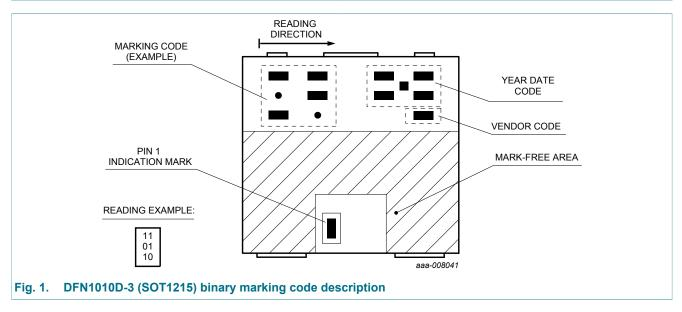
60 V, 1 A PNP low VCEsat (BISS) transistor
