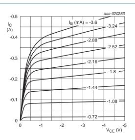
Fig 8. PDTB113EQA: Collector current as a function of collector-emitter voltage; typical values
