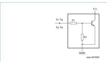
Fig 32. Resistor test circuit
