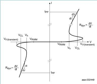
Fig. 3. Transient characteristics for a bidirectional ESD protection device
