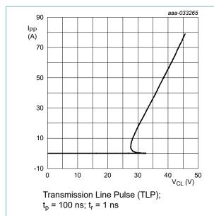
Fig. 5. Dynamic resistance with positive clamping; typical values
