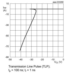
Fig. 6. Dynamic resistance with negative clamping; typical values
