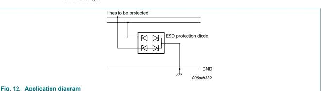
The device is designed for the protection of up to two bidirectional data lines from surge pulses and ESD damage.
