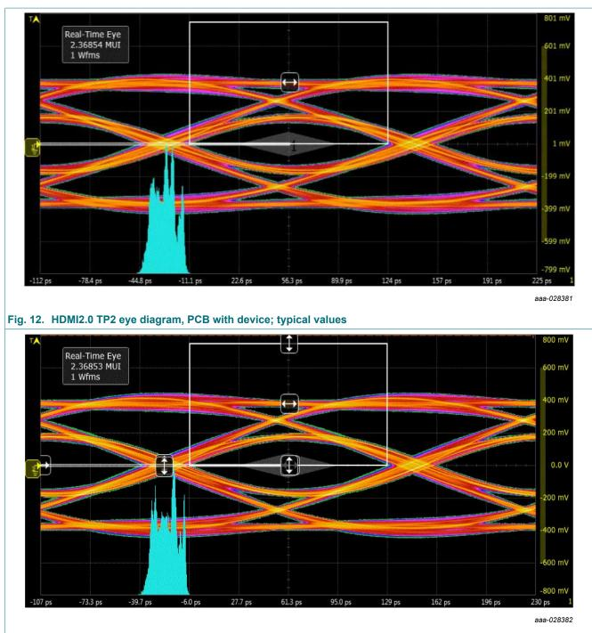
Fig. 13. HDMI2.0 TP2 eye diagram, PCB without device; typical values
