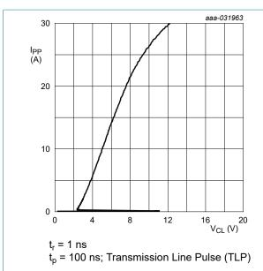
Fig. 5. Dynamic resistance with positive clamping; typical values
