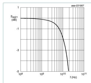
Fig. 3. Insertion loss; typical values
