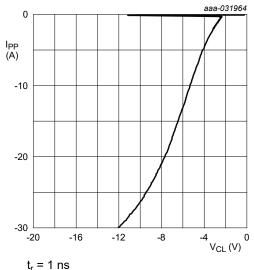
$t_r = 1 \text{ ns}$  $t_n = 100 \text{ ns}$ ; Transmission Line Pulse (TLP)
