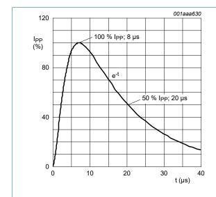
Fig. 1.  $8/20~\mu s$  pulse waveform according to IEC 61000-4-5
