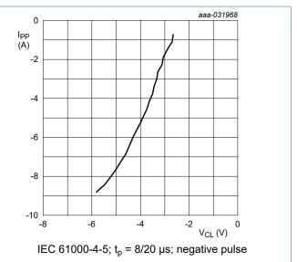
Fig. 10. Dynamic resistance with negative clamping; typical values
