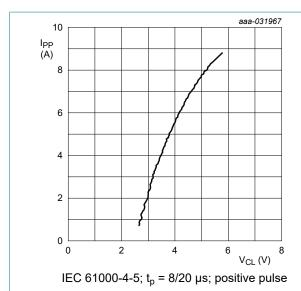
Fig. 9. Dynamic resistance with positive clamping; typical values
