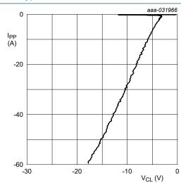
$t_r$  = 600 ps  $t_p$  = 5 ns; Very-Fast Transmission Line Pulse (VF-TLP)
