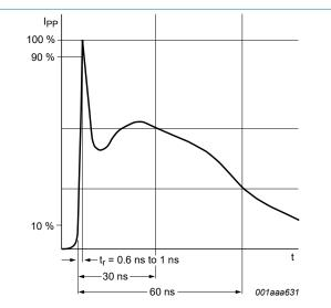
Fig. 2. ESD pulse waveform according to IEC 61000-4-2
