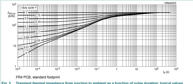
Transient thermal impedance from junction to ambient as a function of pulse duration; typical values Fig. 3.
