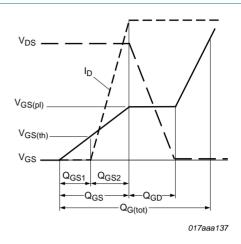
Fig 15. Gate charge waveform definitions
