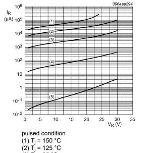
(2)  $T_j = 125 ^{\circ}C$ (3)  $T_j = 85 ^{\circ}C$ (4)  $T_j = 25 ^{\circ}C$ (5)  $T_j = -40 ^{\circ}C$
