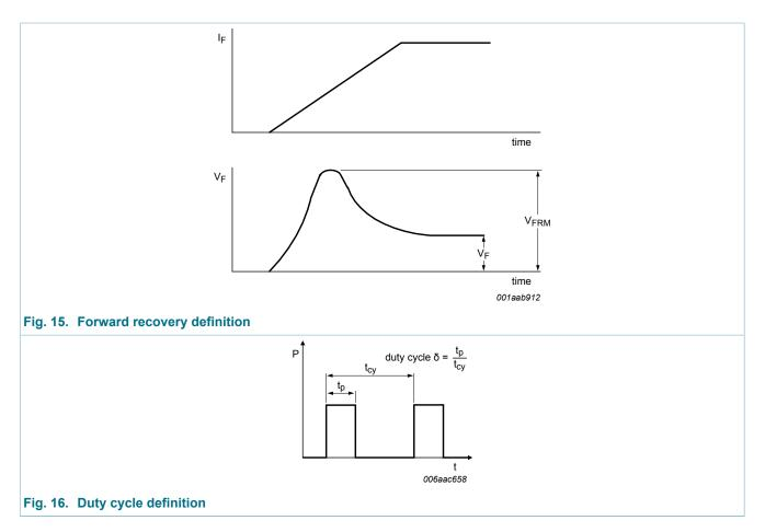
The current ratings for the typical waveforms are calculated according to the equations:  $I_{F(AV)} = I_M \times \delta$  with  $I_M$  defined as peak current,  $I_{RMS} = I_{F(AV)}$  at DC, and  $I_{RMS} = I_M \times \sqrt{\delta}$  with  $I_{RMS}$  defined as RMS current.
