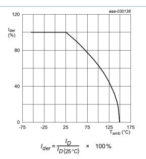
Fig. 2. Normalized continous drain current as a function of ambient temperature
