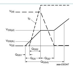
Fig. 15. Gate charge waveform definitions
