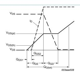
Fig. 15. Gate charge waveform definitions
