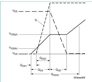
Fig. 15. Gate charge waveform definitions
