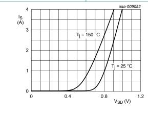
Fig. 16. Source current as a function of source-drain voltage; typical values
