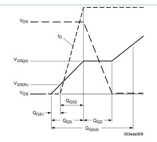
Fig. 15. Gate charge waveform definitions
