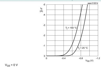
Fig. 16. Source current as a function of source-drain voltage; typical values
