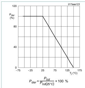
Normalized total power dissipation as a function of junction temperature
