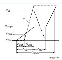
Fig. 15. Gate charge waveform definitions
