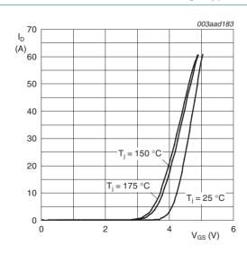
Transfer characteristics: drain current as a function of gate-source voltage; typical values
