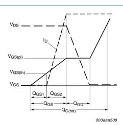
Fig 14. Gate charge waveform definitions
