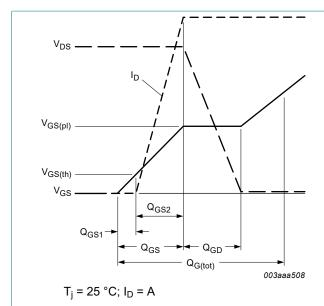
Fig. 2. Gate-source voltage as a function of gate charge; typical values
