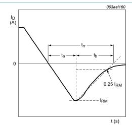
Fig. 3. Reverse recovery timing definition
