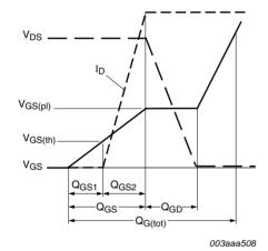
Fig 13. Gate charge waveform definitions
