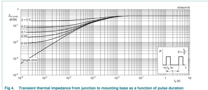
rig 4. Transient thermal impedance from junction to mounting base as a function of pulse duration
