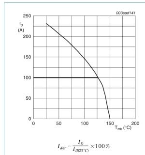
Fig 1. Normalized continuous drain currnet as a function of mounting base temperature
