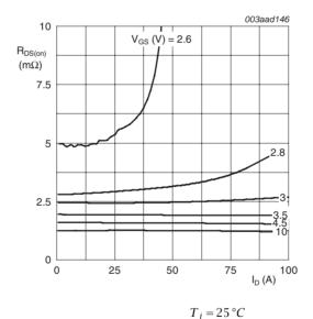
Fig 17. Drain-source on-state resistance as a function of drain current; typical values
