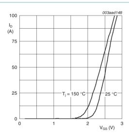
Fig 9. Transfer characteristics: drain current as a function of gate-source voltage; typical valuesvalues
