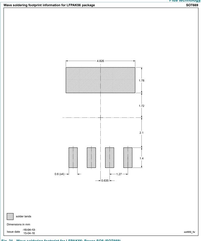
Fig. 21. Wave soldering footprint for LFPAK56; Power-SO8 (SOT669)
