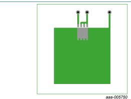
Fig. 6. PCB layout for thermal resistance junction to ambient 1" square pad; FR4 Board; 2oz copper
