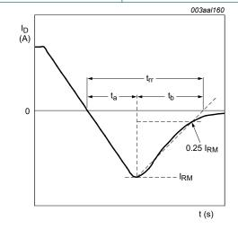
Fig. 18. Reverse recovery timing definition
