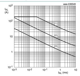
(1)  $T_{j \text{ (init)}}$  = 25 °C; (2)  $T_{j \text{ (init)}}$  = 150 °C; (3) Repetitive Avalanche
