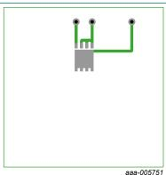
Fig. 7. PCB layout for thermal resistance junction to ambient minimum footprint;FR4 board; 2oz copper
